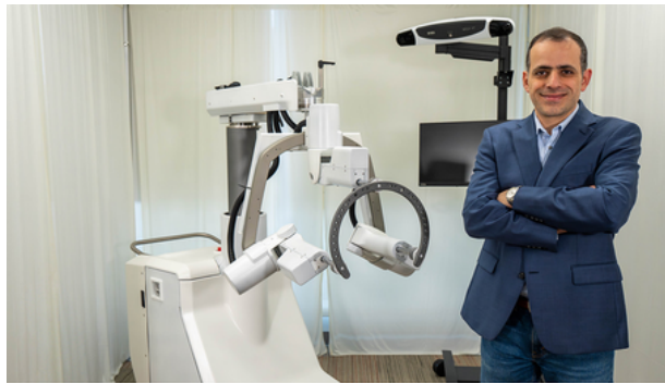
Mohammad Abedin-Nasab, an associate professor of biomedical engineering at Rowan University, stands with Robossis Alpha, the world's first robotic surgical system designed for minimally invasive alignment of fractured long bones.
